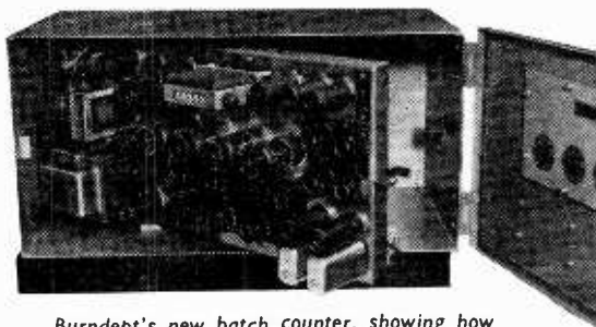
Burndept's new batch counter, showing how the chassis swings out for servicing.
